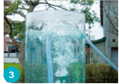
Sludge stirred in the cylinder churns in a spiral and circulates in the tank for purification.
